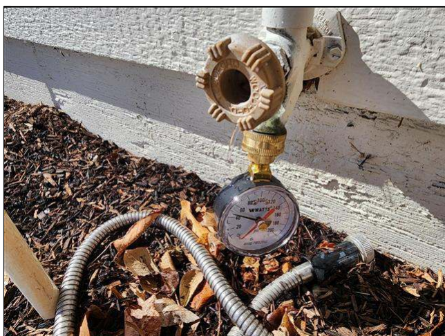
5.2 Item 5(Picture) water pressure at front hose bib
