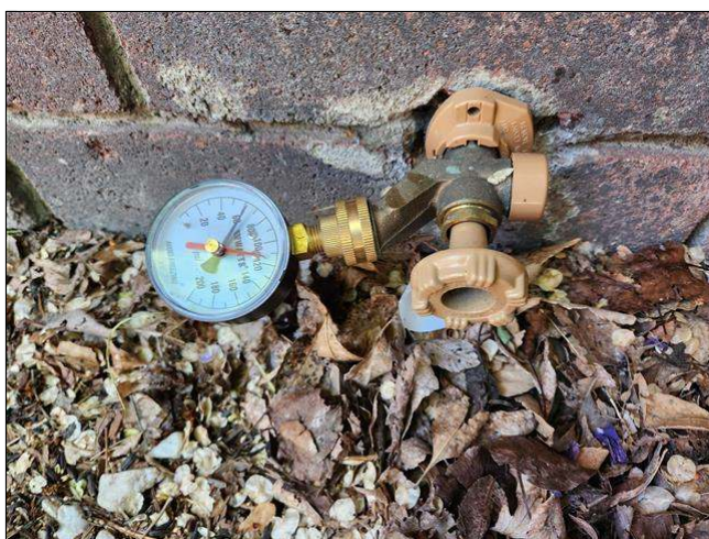
5.1 Item 3(Picture) water pressure at north hose bib
